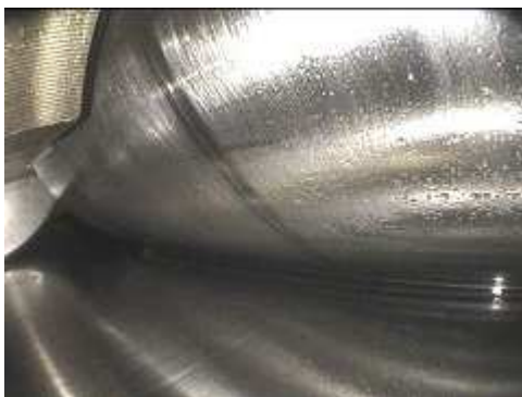
Figure 5: Using lenses with a high depth of field allows inspectors to inspect large or deep spaces more quickly.
