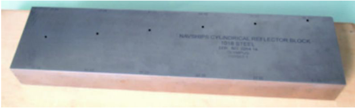
Figure 15: A Calibration Block for UT Inspections
