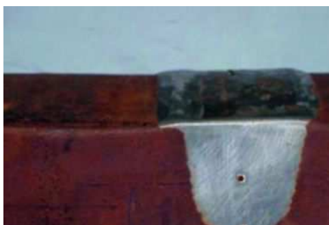
Figure 1: Welding of Cladded Pipes
