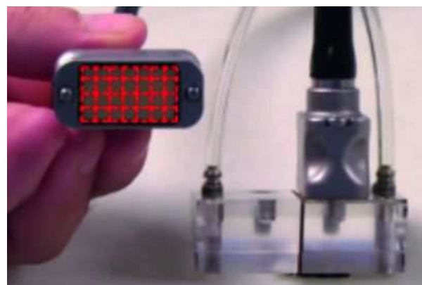
Figure 6: A Wedge Holding a DMA Probe
